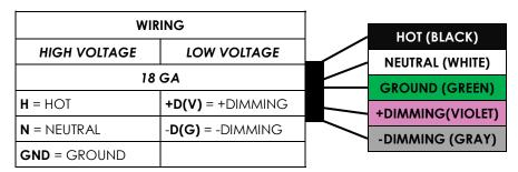
This wiring diagram is showing a standard set of wires for a basic fixture.
