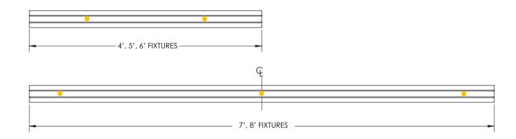
NOTE: Hole size at mounting locations is Ø.266".
