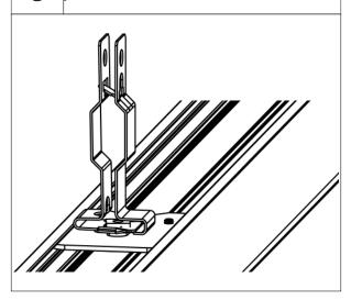
Attach appropriately rated cable though hole and secure cable to structure.
