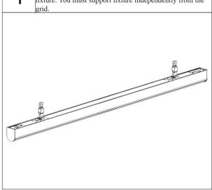
Attach independent support clip (caddy part 3 IDS or IDS9) to 15/16" or 9/16" t-grid by folding two halves of the support clip around t-grid. Lock the two halves together when support clips are in desired location.
