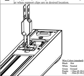
Attach fixture to support clip by sliding bracket located on top of the fixture over washer on support clip and lock in position with set screws.
