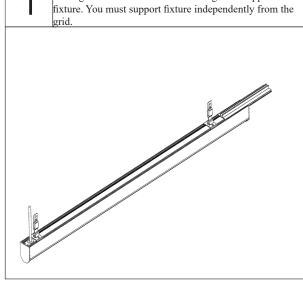
Attach independent support clip (caddy part 3 IDS or IDS9) to 15/16" or 9/16" t-grid by folding two halves of the support clip around t-grid. Lock the two halves together when support clips are in desired location.
