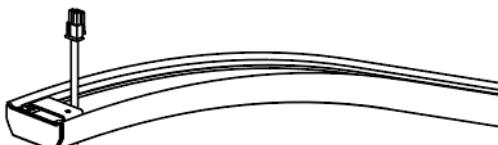
Low Voltage power plug is on one end. To be plugged into the low voltage power wire from the driver box. Install a J-box behind the fixture. Drill a small hole through the substrate to push the plug through for installation.
