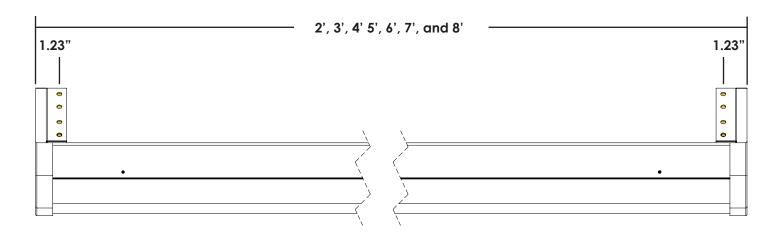
Hole located in the endcap for power and DMX input (Made for Standard Conduit fitting )
