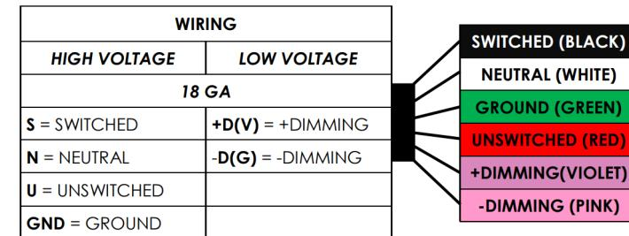
This wiring diagram is showing a set of wires for a fixture with an emergency battery.
