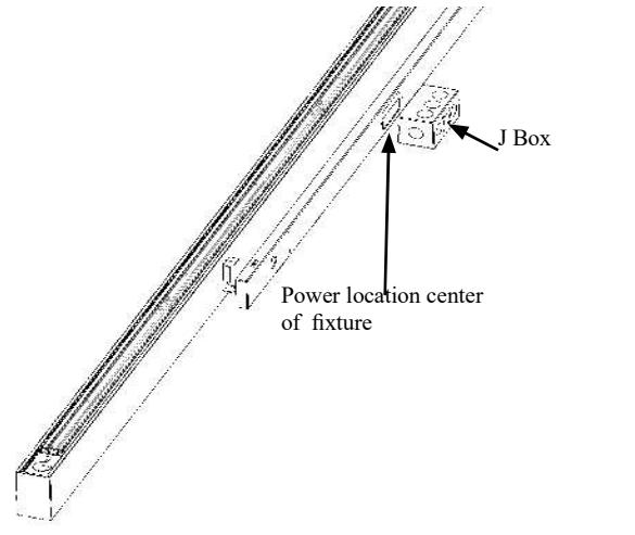
**2** Remove wall mount bracket from fixture. Secure bracket to structure in desired locations.
