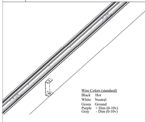
**4** Use slots to center and secure fixture.
