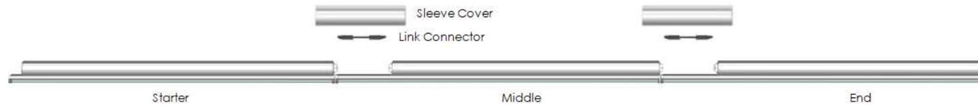
Each run of StarLink includes a starter and end fixture. Runs over 12' or 16' will include middle fixtures to build the run to the requested length. Each middle and end fixture includes a link connector and our proprietary sleeve cover. This sleeve cover ensures straight runs at any length.
