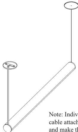
Note: Individual fixture will come with aircraft cable attached. Mount fixture to the structure and make the proper connections. The mount height is adjusted at the canopy
